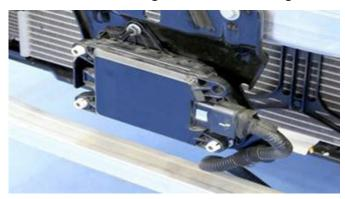
This system is designed to avoid front-end impacts or at least help reduce the severity of an impact by decreasing the vehicle speed. This system uses radar sensors to detect the relative distance and the changing speed of the traffic ahead, and it can automatically brake if an imminent collision is detected. In addition to the damage of the radar sensors, a forward-collision can also affect the suspension and damage the brakes. This obviously will require ADAS systems to be calibrated.
