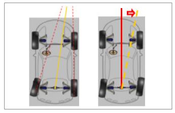
The thrust line define the vehicle driving axis, so the thrust angle value have to be inside the VM range to guarantee the right direction of the vehicle.
